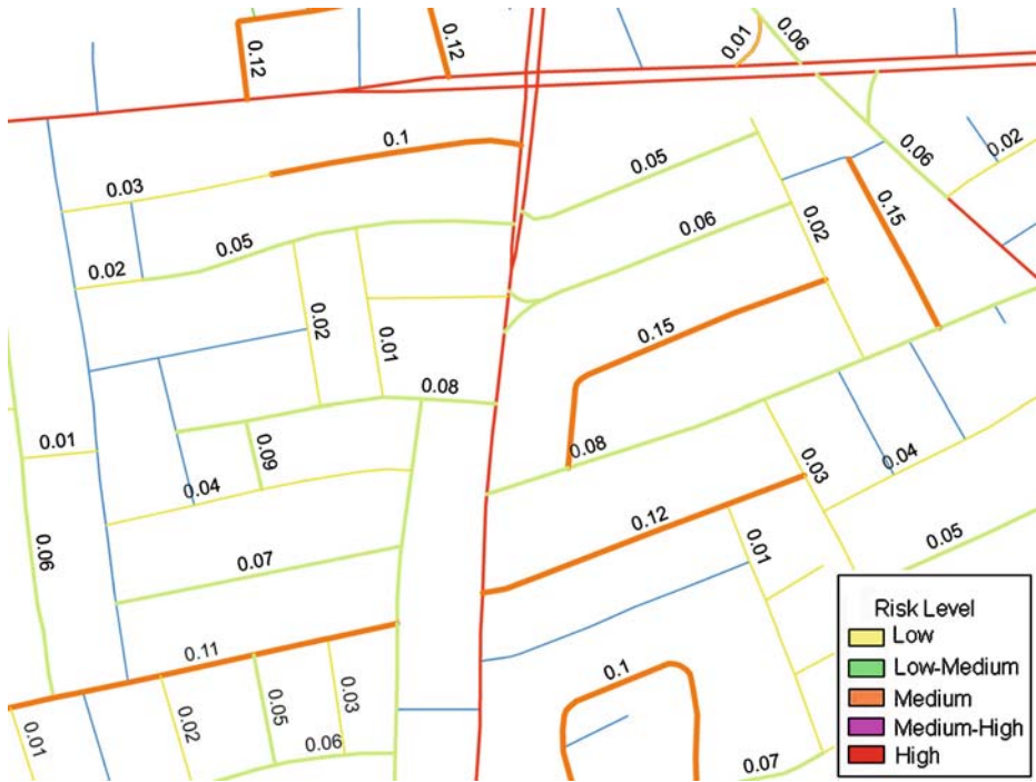
Fig. 11 Risk-of-failure analysis mapping at street level (colour variations indicate varying degrees for risk-of-failure)
